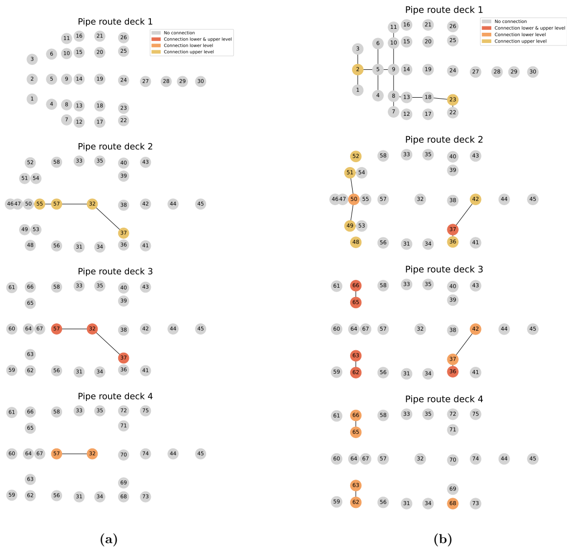
Figure 10: Optimal RO pipe route for the realistic graph. Figure 10a shows the single-walled pipe route, whereas Figure 10b represents the double-walled pipe route.
